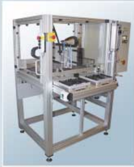
Automatic silicone gasketing dispensing with x-/y-robot
